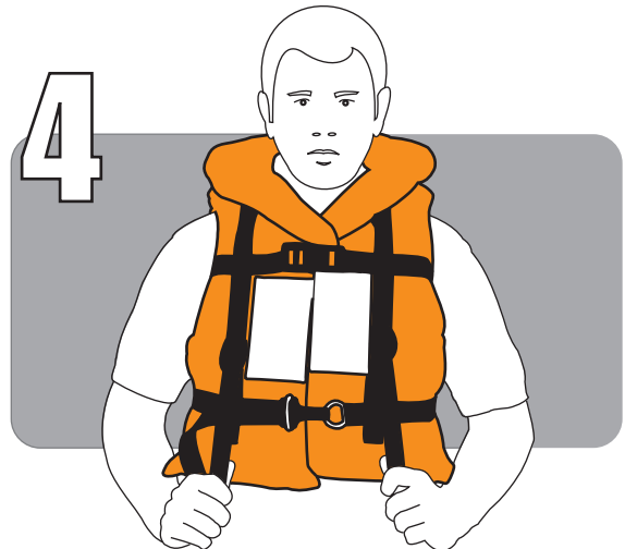
GRASP FREE END OF SUSPENDER WEBBING AND PULL DOWNWARD UNTIL SNUG
